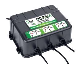
With 3 channels available, the FULBANK 2000 diagnoses, charges and maintains batteries from 4Ah to 40Ah (120Ah in maintenance). This 6V-12V bank charger is compatible with lead-acid (Gel, AGM, MF, Dry, Ca/Ca, Wet) and Lithium (Life-PO4) batteries.
